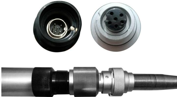
\* Designed and manufactured according to the oil logging process instruments and equipment, with positioning pin, two axial seals, high pressure and high temperature resistance, connector can be exchanged for the use of different diameter probes.
