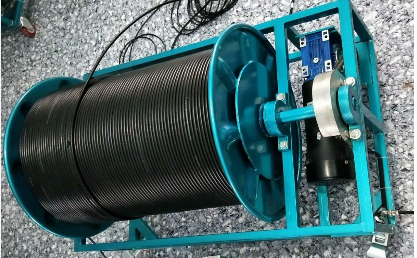
The electric winch
