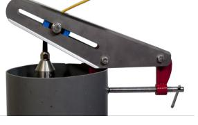
TEL-906-000: 90° VIEW OPTION → with and without vertical centering device TEL-907-000 (from 80mm to 260mm diam.)
